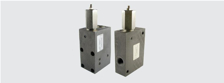
HYDAC accumulator charging valves control, within an adjustable switching range, the charging of the accumulator. By combining the charging valve with an accumulator, pumps and motors on hydraulic plants with fluctuating flow requirements can be sized smaller. This saves costs and energy - thus preventing unnecessary heat development.
